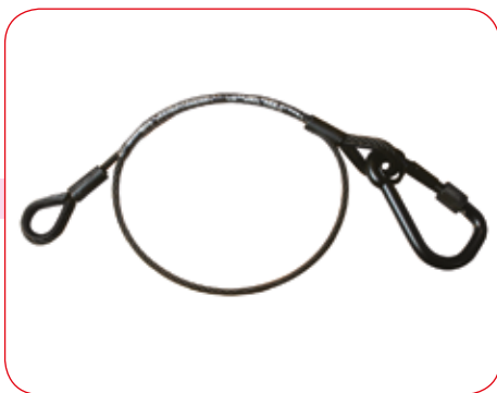
Safety Bond WLL 36kg - 600mm T2844001 4mm wire
